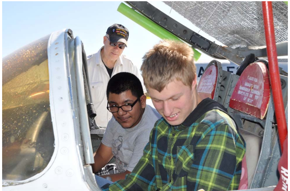
Experiencing the cockpit of the T-37 Tweet. The instructor sat on the right, the student on the left. Though small and unglamorous, the Tweet is possibly our most popular climb-aboard aircraft because it is low to the ground and easy to climb into, which is great for those with reduced mobility. It's also easy to understand: just move the control stick and you can see the ailerons and elevator move!
