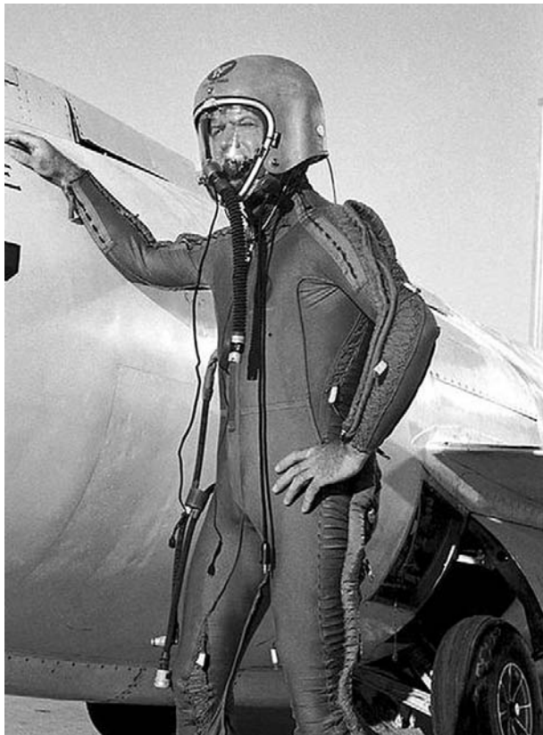
An airman in a partial pressure suit similar to the one fitted to C J. Under low pressure, the cords along the seam lines tightened up, squeezing the person and creating artificial pressure. Apparently they worked, though C J never actually flew in one.
