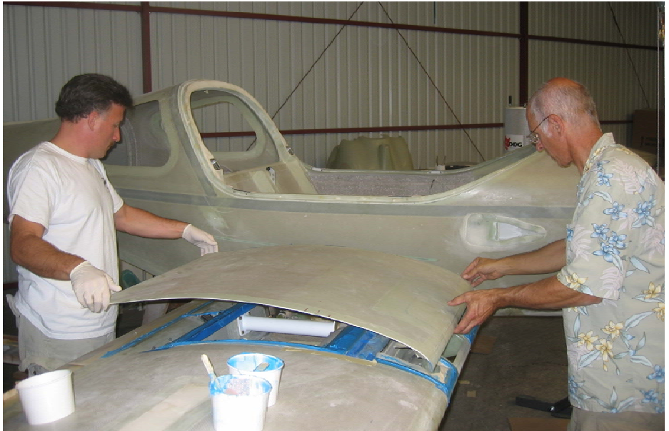
Andy (at right) installs an upper wing panel on his first Lancair with the help of award-winning Lancair builder Don Barnes, at the Lancair factory shop in Redmond, Oregon. If you build over 50% of the plane yourself, the FAA considers it a homebuilt.
