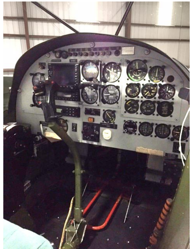
The SM-1019 cockpit and instrument panel.
