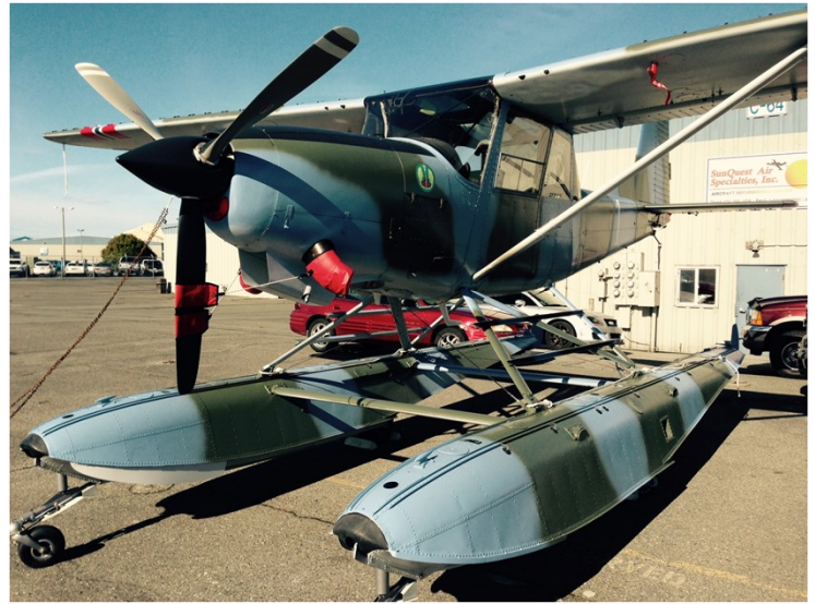
Our L-1019. Note the wheels that retract into the floats. So one could take off from the concrete runway at the airport, fly to Lake Berryessa, land on the water, have a swim and a little lunch, take off again, and land back in Santa Rosa.
