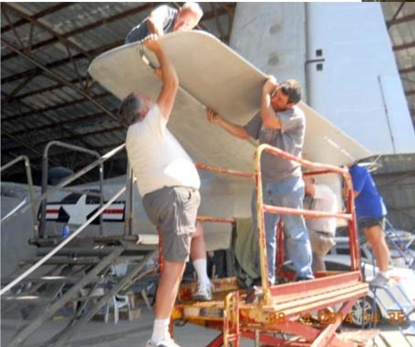
Top right: Cody sets up the elevator for installation.
