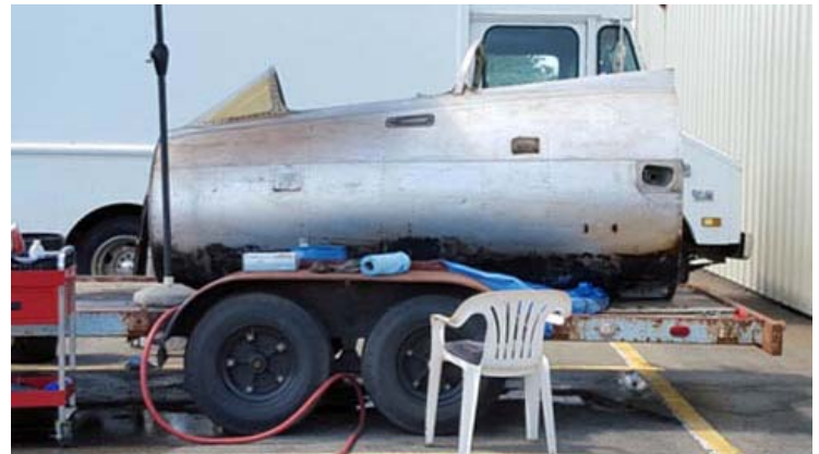
The L-29 Delfin cockpit section in the outdoor "workshop", as its ancient coat of peeling paint is being removed.
