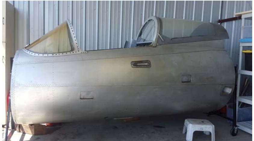
The L-29 Delfin cockpit section that will house the simulator. This is it after the old paint has been stripped off.
