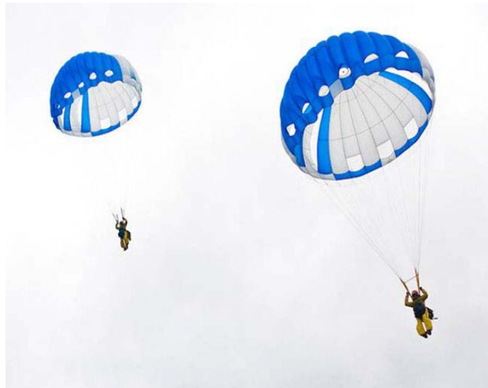
The Smokejumpers use advanced round canopy parachutes, but will be switching to square airfoil 'chutes within 3 years.
