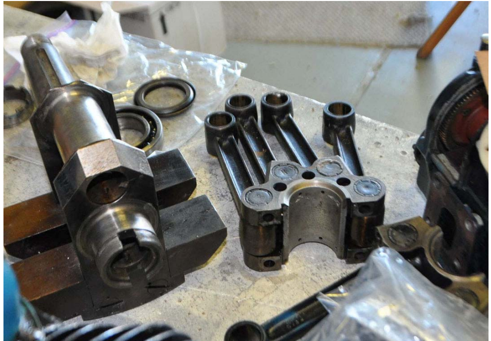
At left is the crankshaft, To its right is one half of the R&AS containing four slave rods. Here, towards the upper edge, the damage is clear. See the inside of the bearing facing the camera. The other half, containing the master piston rod and two slaves is obscured by the plastic bag at lower right, and that bearing surface is not pristine.
