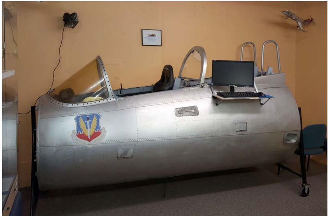
The new 3D Flight Simulator in place in the Gift Shop. This is the actual nose section of an L-29 Delfin jet trainer. It doesn't move around on hydraulics like state-of-the-art flight simulators used by the military and commercial schools, but the overall experience is remarkably good.
