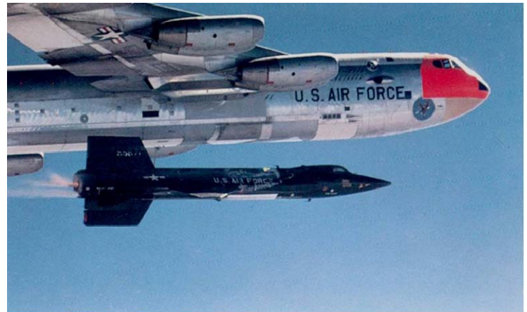
An X-15 with the later, larger engine (note single rocket nozzle) is launched from the B-52 mother ship. .
