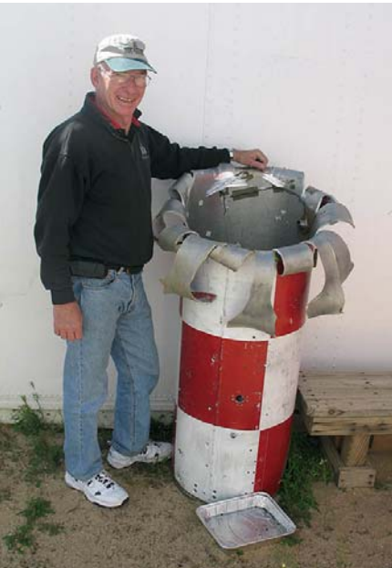
CJ and the first test canister. The shroud lines failed and the canister fell like a bomb.
