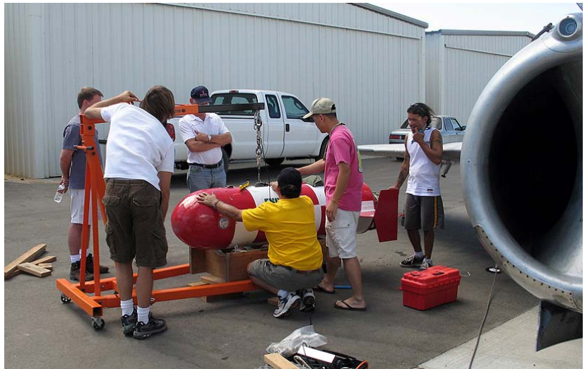
The FNC crew loading a test canister onto the MiG at California City. FNC was the military contractor developing the recovery system. The gaping black maw at the right is the MiG's air intake.
