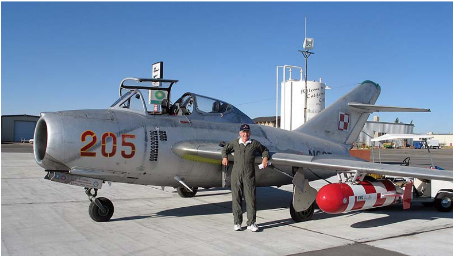
CJ Stephens with the MiG-15 UTI he flew to test parachutes for the Navy's BQM-74 Target Drone. That's a test canister under the left wing.
