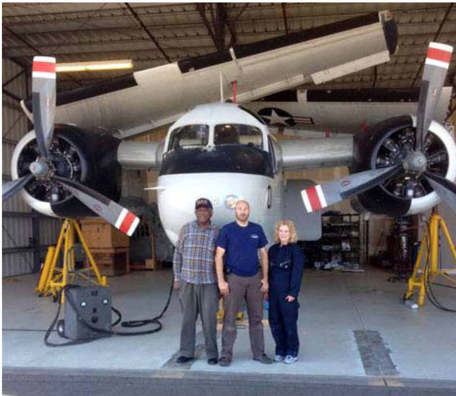
Look Ma, no wheels! The C-1A in the midst of its gear swing test. The plane is supported 100% on jacks, and the landing gear is fully retracted. From left to right: Henry Granger, Chris Brown, and Air Show Director Nancy Heath.
