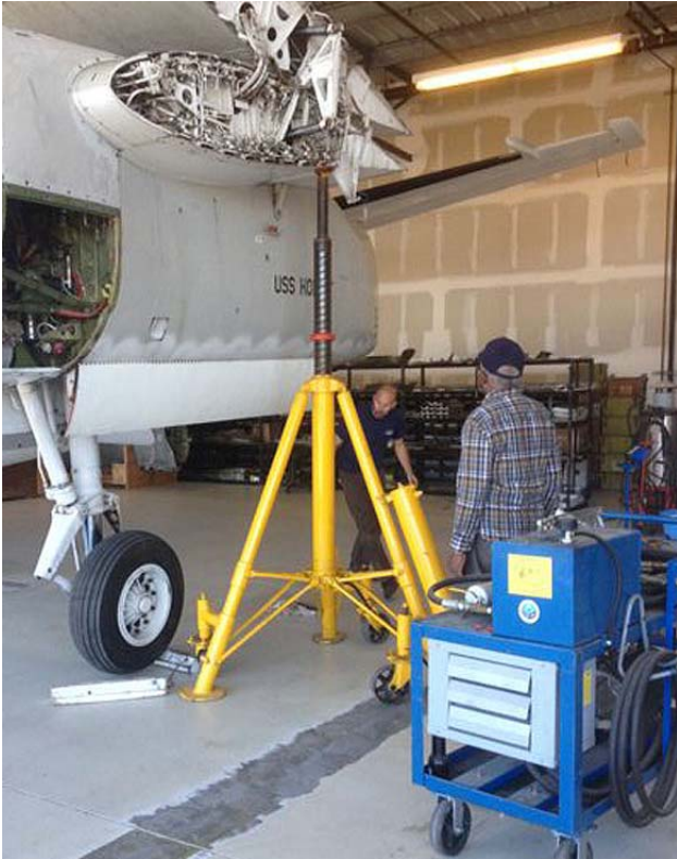
Henry Granger (front) and Chris Brown (rear) check that the plane is properly jacked up in preparation for the gear swing test.
