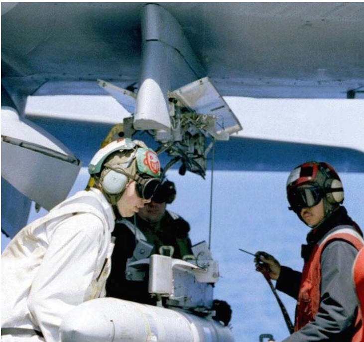
A Navy crew installs a LAU-118 HARM Missile Rail on an EA-6B Prowler. Two such rails are slated for PCAM. See story at right.
