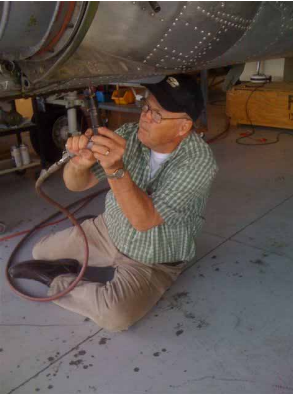
Don Davis, aircraft mechanic extraordinaire, re-works some of the riveting on PCAM's T-28C.
