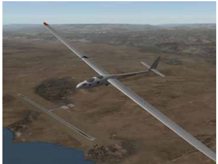
Computer-generated image of Perlan II. Note the ultra-streamlined but low-visibility cockpit. An onboard video camera will help with landings.
