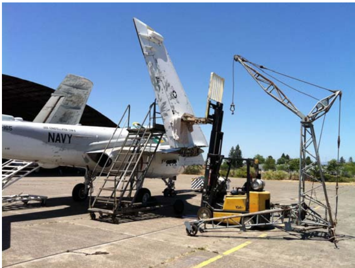
Work proceeds apace on the Intruder's weapons racks, Summer 2013. Note the badly peeled paint from years sitting in the sun.
