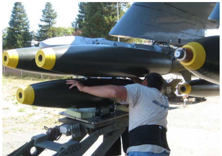
Work proceeds apace on the Intruder's weapons racks, Summer 2013. Note the badly peeled paint from years sitting in the sun.
