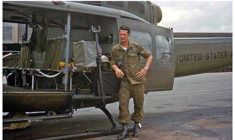
Above: Bob stands next to his position on the aircraft. His machine gun is to his right, pointed down. His right elbow is resting on one of the extra-large ammo cans the crew installed.
