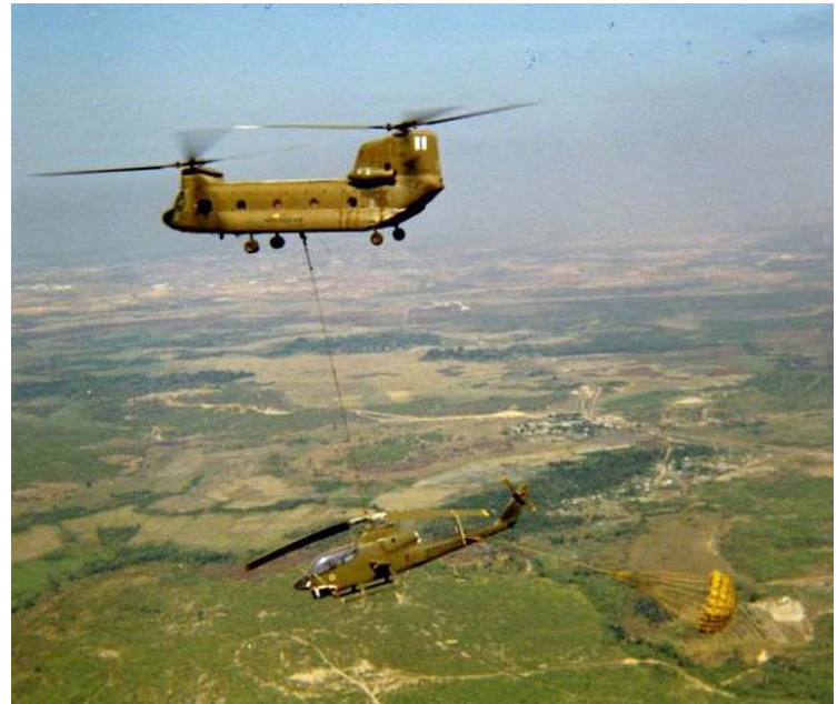
Above: Recovery. A Chinook carries a damaged Cobra gunship. In lower right you can just make out a drag parachute which was attached to the wreck to keep it from spinning in flight. Chinooks were used for heavier loads like this one. The countryside in the background is typical of the parts of Vietnam where Bob served.
