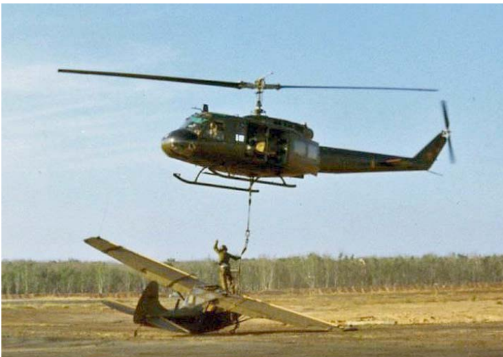
Above: Recovery. A Huey hovers over an O-1 Bird Dog that made a bad landing back at base and collapsed its landing gear. A lifting harness has already been attached to the damaged plane and the man on the wing has attached the Huey's lifting strap to it. Few recoveries were this safe; many were made under fire or in areas that had just been cleared of enemy soldiers. The first recovery helicopter to the scene would perform dustoff, which was the rescue of wounded soldiers or aircrew. The second chopper would recover the downed aircraft or other equipment. Bob's job as Door Gunner was to shoot back at the enemy if the recovery ships came under fire.
