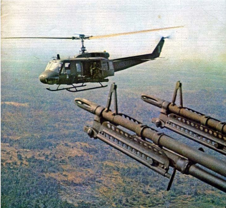
Above: the Door Gunner's view and his guns. For a while, they tried increasing firepower by doubling up the M-60 machine guns as seen here, but it did not work well so they returned to singles.
