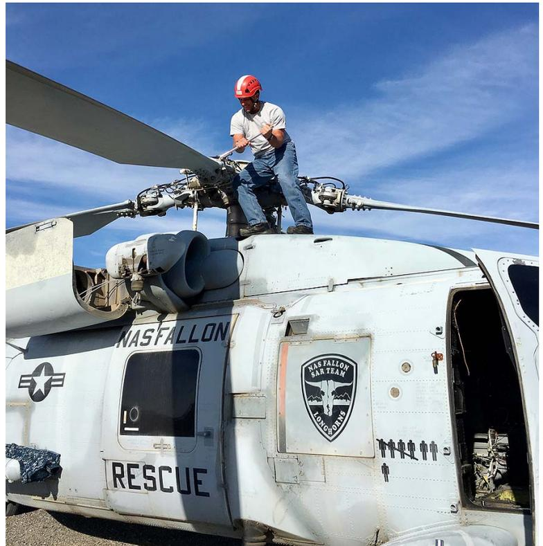
Mark struggles in the Nevada heat to remove a bolt securing a rotor blade. As he worked, he got to watch (and hear) F/A-18 Hornets practicing nearly right overhead. This aircraft is on loan from the National Naval Aviation Museum at Pensacola, Florida.
