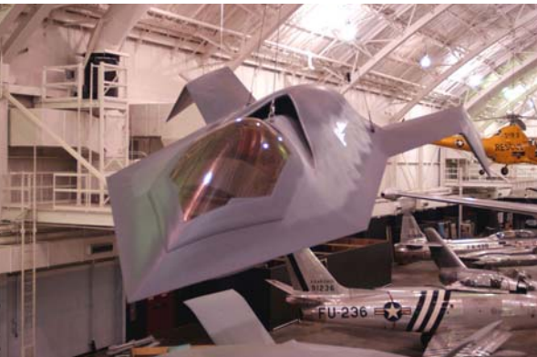
The Bird of Prey was named after Klingon ships from the Star Trek series. Only one Bird of Prey was built, as a test bed for stealth technology.
