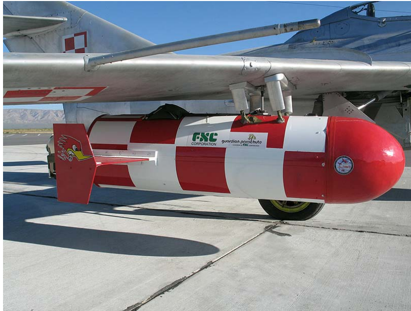
The test canister mounted on the MiG. The MiG was a good aircraft for this because of its speed and built-in hard points designed for carrying heavy, droppable loads.
