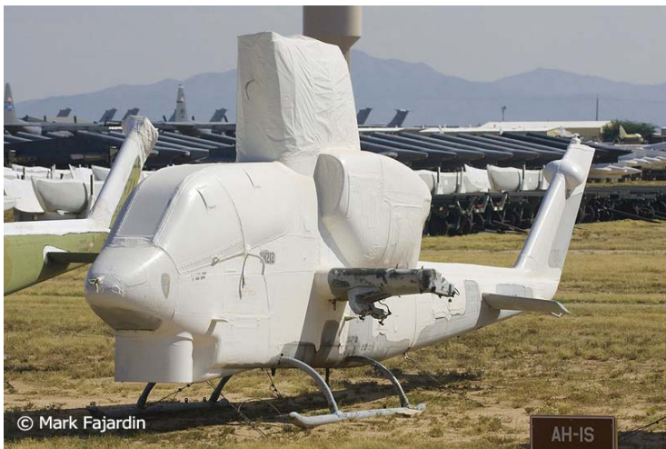
This AH-1J Sea Cobra at AMARG Tucson is slated for PCAM, if we can get the funds together for de-mil and transport to Santa Rosa. She's shown wrapped in white protective materials.
