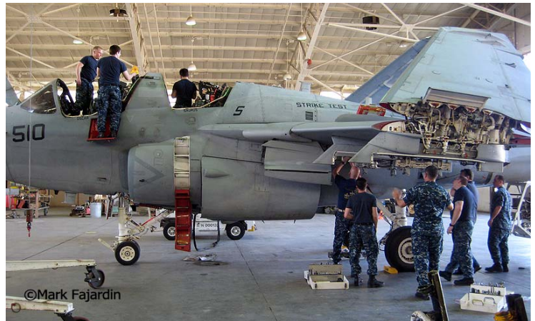
The honorably retired EA-6B Prowler #160436 during "de-mil" at Castle. Demilitarization means the removal or disabling of all military equipment such as ejection seat charges, engines, etc.
