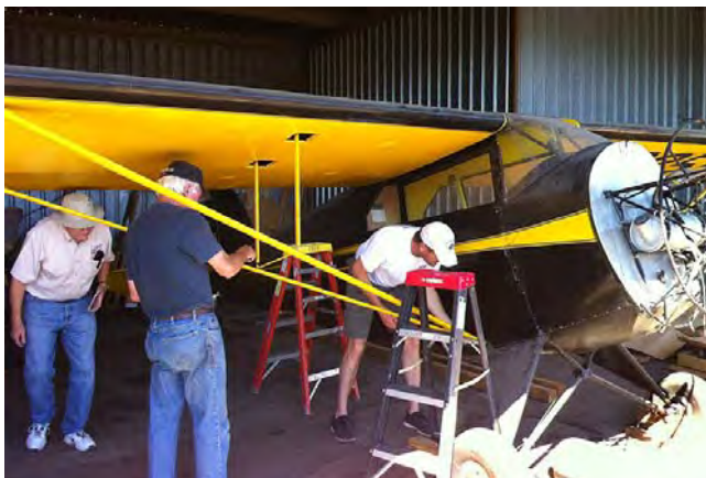
The crew starts removing the wings. They were carried home on the rack on the back of a pickup truck.
