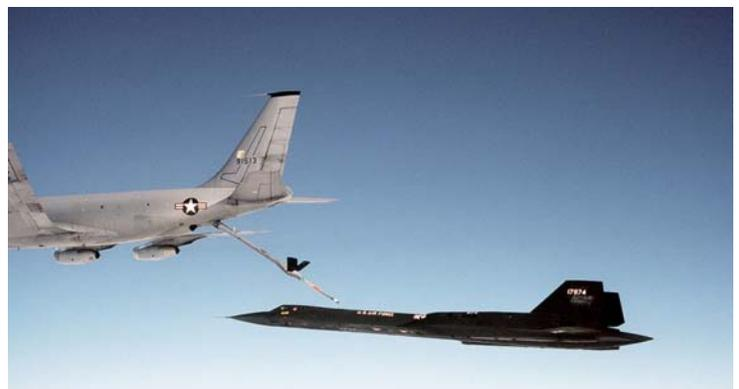
The first thing an SR-71 pilot did after takeoff was refuel. The tanker would fly at about 300 knots, but the SR-71 stalled at about 290, leaving a very small margin of error. Hooking up was a slow process, and extremely difficult at night in bad weather.
