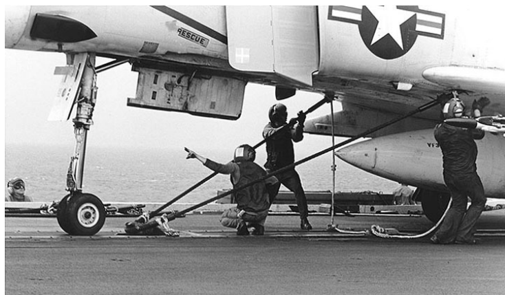
The launch bridle (diagonal black lines) is clearly visible as this F-4 Phantom is readied for launch (U.S. Navy Photo)
