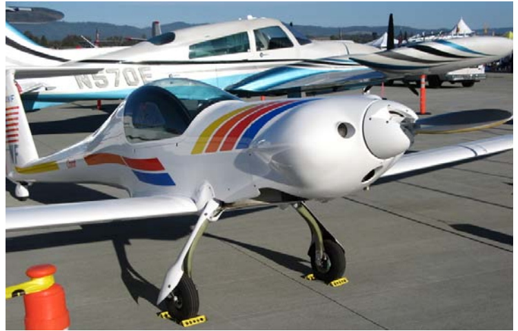
This 2007 Carat is a powered sailplane, with a propeller that folds forward to reduce drag when the engine is off. This and several other high-tech and lightweight planes were seen in the static display section. There was also a booth staffed by members of the Santa Rosa Chapter of the Experimental Aircraft Association (EAA), who were more than willing to talk about the advances in civil aircraft engineering and avionics that can make flying far more affordable and accessible. Several LSAs (light sport aircraft) were on display. LSAs are a great way to join the world of flight.
