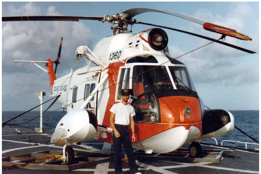
Wayne and an H52 in the Caribbean. Note the single engine. The grid of 4x4 timbers on the deck was a primitive but effective chocking system.
