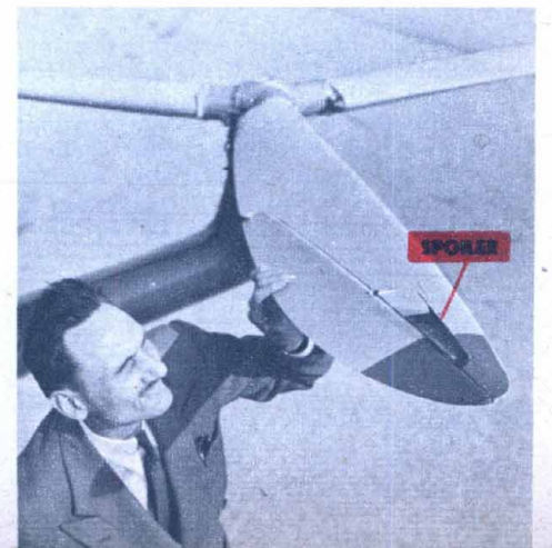
Inventor-designer Landgraf, below, checks the "spoilers" and ailerons on the tips of the rotor blades. They provide directional control. The automatic pitch control, left, allows the pilot to concern himself only with maneuvering the stick, the throttle and the foot pedal.
