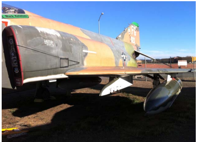
Tony Sarganis and Ron Stout installed the MAU-12 bomb racks on November 2. Now we just need some ordnance to put on them.
