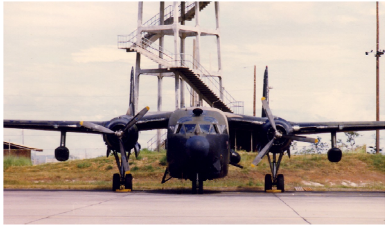
AC-119K "Stinger". The pods hanging from the wings are jet engines. The dark protrusion on the plane's port side is radar. Just under the radar you can see one of the two 20mm Vulcan cannons.
