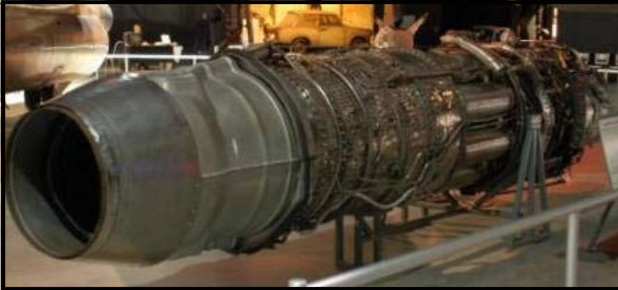
Like the [Allison J33](#) centrifugal jet engine, the Allison J35 was based on a General Electric Design. It was developed by the General Electric company alongside the Whittle based J33, and was the first Axial-Flow jet engine to be used by the USAF.
